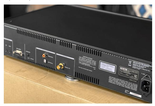
Before we get there, though, a quick peek at the back panel. Not a lot to talk about here, given that this is a CD transport and not a CD player. You have your choice of optical or coaxial digital outputs, as well as an input for TEAC's optional CG-10M 10MHz master clock generator. Also, slightly out of focus on the left, there's an RS-232 port for advanced control systems, as well as a 12V trigger input and output.
